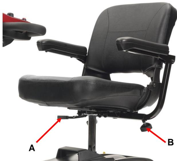
A. Seat Swivel Lever – Lift upwards to rotate your seat. The seat will swivel to the left or right with locking positions each side at 45° intervals.
