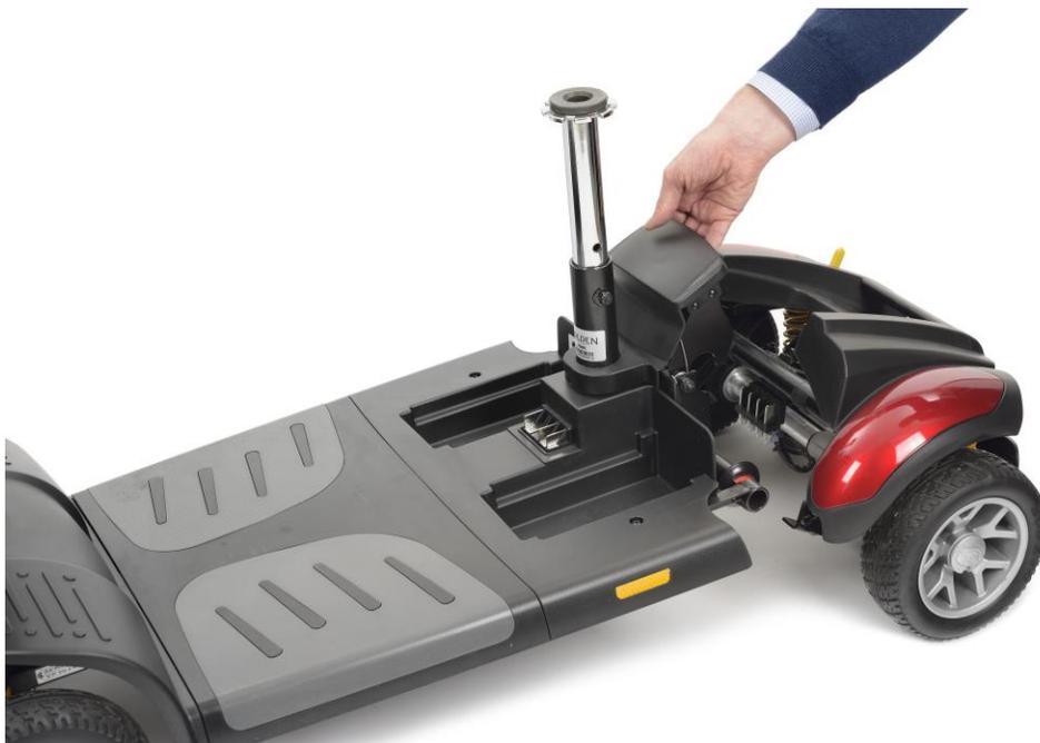
4. Fold down your tiller by placing one hand on the tiller handle and with the other rotate the hand wheel located at the bottom of the tiller anti clockwise. Once the tiller moves freely you can move it all the way down and turn the hand wheel clockwise until it is tight and holds the tiller in place.
