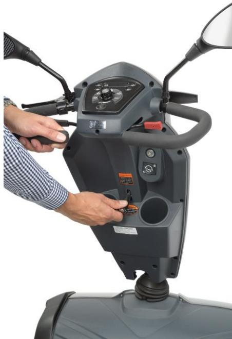
If you'd like to adjust your tiller simply push down on the adjustment lever until the top part of the tiller moves freely up and down. Once the tiller is in the correct position just let go of the lever.
