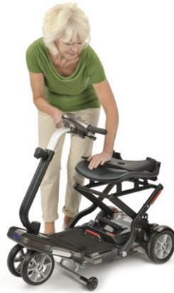
4. Finally push the tiller against the seat and the front of the floor pan towards the rear wheels to ensure your scooter is locked into the folded position.
