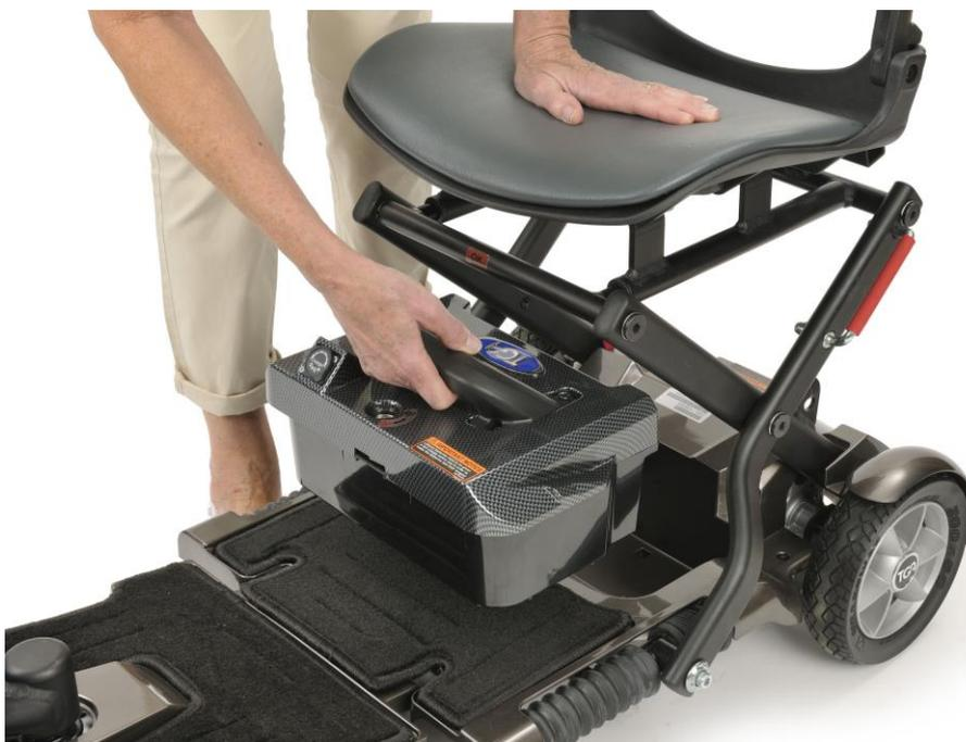
To remove the battery pack first ensure the pack is unlocked by inserting the key into the pack and turning it 90° anti clockwise to the unlock position. Then simply lift the pack up away from the base of the scooter and the seat using the handle provided.
