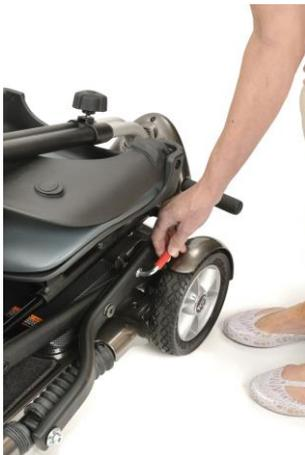
2. Pull the tiller away from the floor pan until the front wheels of your scooter touch the floor.
