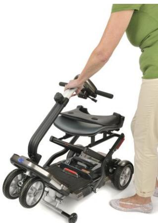
3. Ensure your scooter is locked in the unfolded position by pulling the seat away from the floor pan with one hand and pushing the tiller away from the seat with the other until you hear a click and feel your scooter lock into this position. Once your scooter is locked in position you will no longer be able to move the tiller towards and away from the seat so use this as a simple test to find out if your scooter is locked in the unfolded position.
