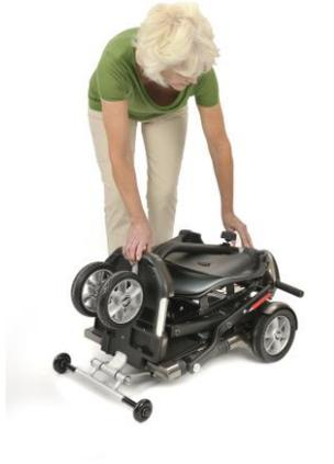
Once folded you can then lift your scooter using the handle at the rear and stand it on its front wheels to move around in the folded position.
