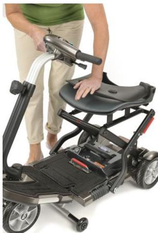
3. Use one hand to push the seat down towards the floor pan and the other to move the tiller towards the seat which will lift the front wheels off the floor and fold your scooter.
