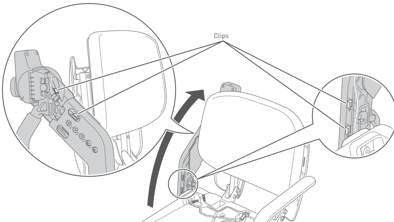
6. Pull out the cable from the cable-threading hole on the seat assembly and arm, then lower the arm.
