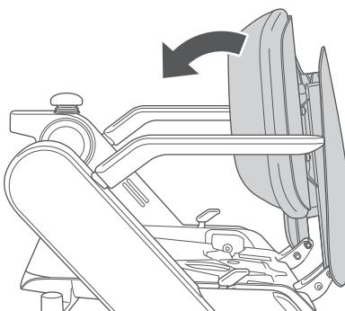
4. Remove the two back support adjustment bolts with the specified tools.
