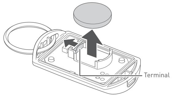
3. Pull back the terminal and install a new battery under the rib in the battery case.
