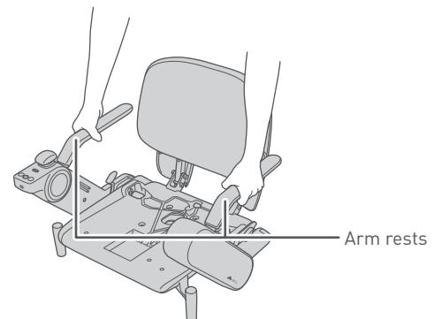
3. Fit the seat assembly straight into position while checking the seat post position from the view hole in the seat assembly.
