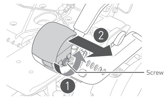
**9.** Attach the round unit at the head of the arm that was removed in Step 8 to the opposite arm.
