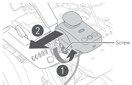
8. Remove the round unit at the head of the arm on which the control pad is not attached.
