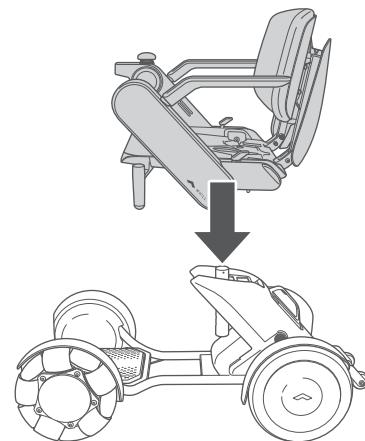
4. Lower the seat release lever so that it is perpendicular to the seat.
