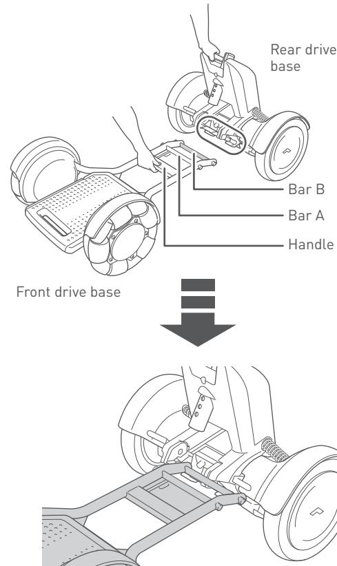
2. Slowly tilt the rear drive base forward and connect the front drive base and rear drive base.
