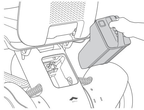
3. Insert the battery straight and press it until it clicks. When it is difficult to insert the battery, push it from the front with force.
