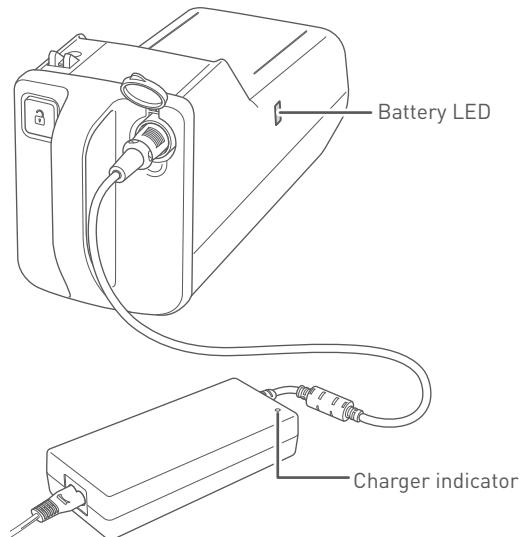
**7. Charging is completed when the charger indicator and battery LED turn green.**
