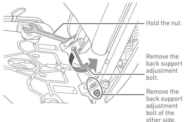
5. Insert the two back support adjustment bolts into the desired holes.
