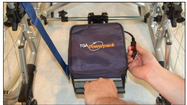
Fig 7 Fitting and Connecting Battery
